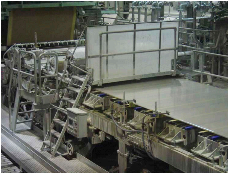
Wire section with a dandy roll PM Lachendorf/Germany
